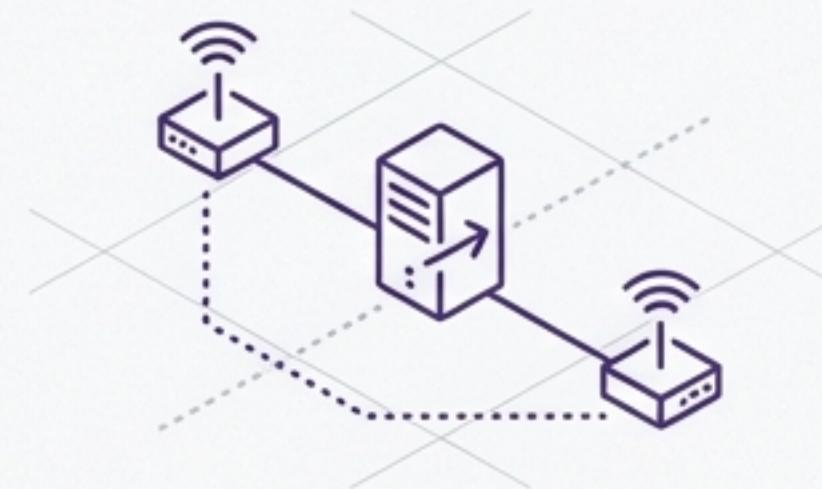
The architecture is designed to establish direct peer-to-peer connections for maximum performance. When firewalls prevent a direct link, the system automatically uses a self-hosted relay server to ensure connectivity is never lost.
